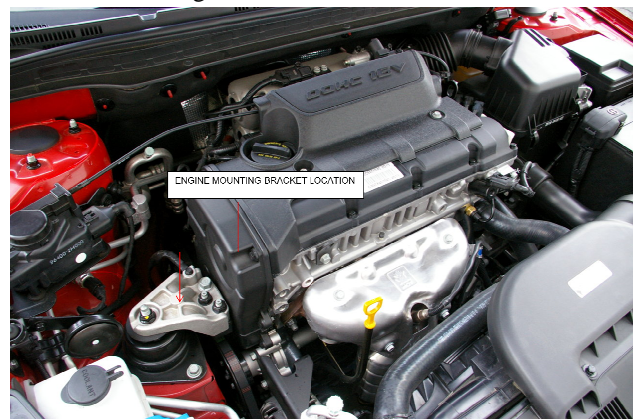
Fig1: Location of engine mounting bracket of a car
